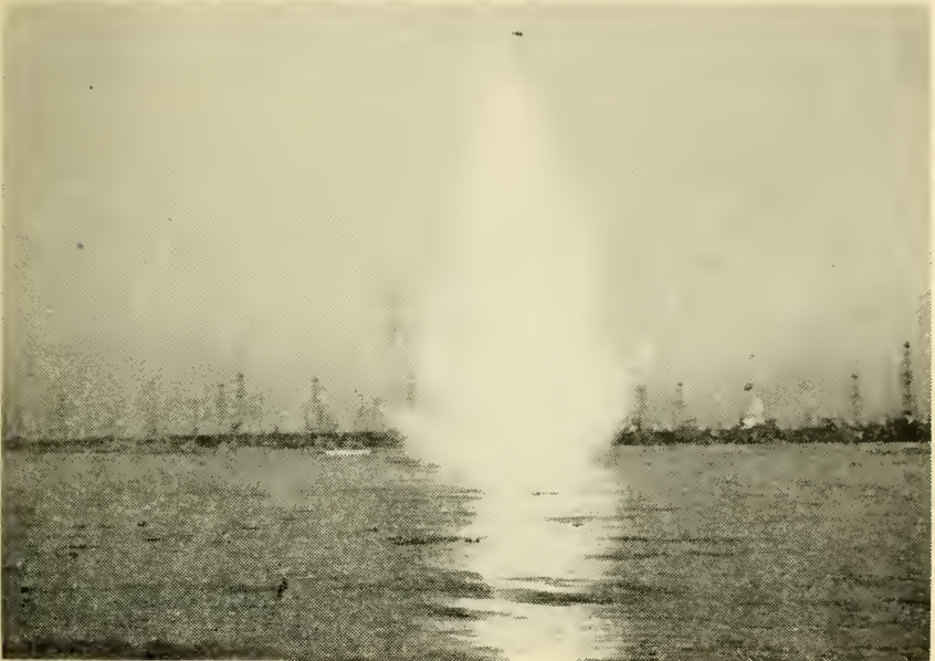
FIGURE 4. Explosion of twenty pounds of dynamite fired four feet below the surface. Dark object above column of water is the float used to buoy the charge.
